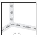
2. Apply a coating of ARDEX WPM 155 Rapid Plus to the entire area to be waterproofed using a brush or roller, a medium nap (8–12mm pile) or 50mm long bristle paint brush is recommended. This first coat should be applied at 0.5mm (wet film thickness) to provide a 0.25mm dry film thickness. Allow to dry. Dry time is approximately 1-2 hours at 23°C and 50% relative humidity.
