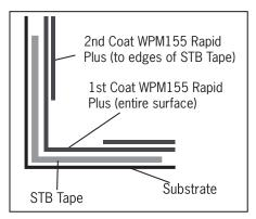
Tiling can begin once the second coat has dried which is generally 3 hours at 23°C in undertile applications. Drying times will vary depending on humidity, surface temperature and porosity of substrates.
