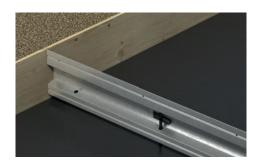
Adjust the key joint to the correct height and secure by tapping in the supplied wedges. If capping strips are to be used allow the appropriate set down distance and apply capping strip prior to pouring concrete.
