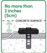
Install the transmitter on rebar no more than 2 inches (5cm) from concrete surface
