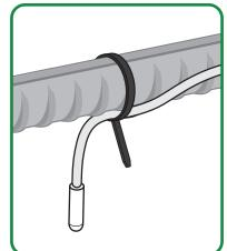
6 Secure the cable and temperature probe below the rebar
