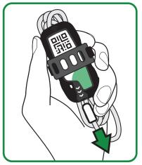
Remove the temperature probe from the sensor to activate
